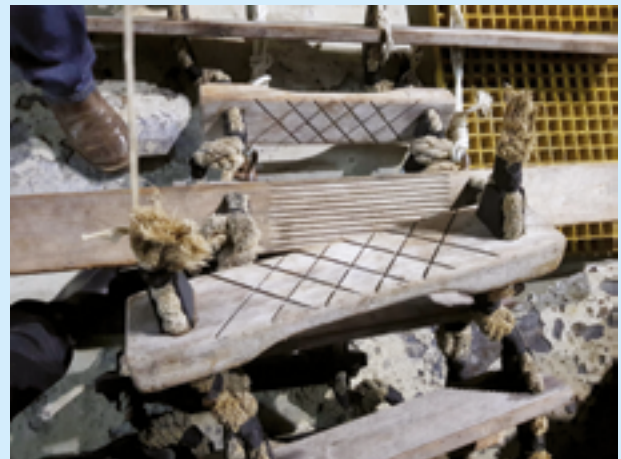
Deathtrap – pilot placed his weight on this ladder prior to disembarking and both side ropes parted!!
