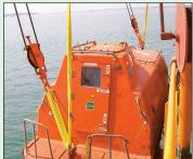
It is important that FPDs are made of resilient material that can absorb shock. In the photo the same principle has also been applied to the hanging-off pennant. This ensures any failure of the hooks would not induce a large shock loading, which in a wire or chain could cause the latter to sequentially fail as the materials have limited resilience. Furthermore, as can often be found in incident reports, corrosion in wires can be present and could cause weakening of wire strops.
