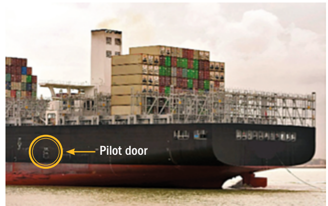
The pilot door not lying within the parallel mid-body in light condition
