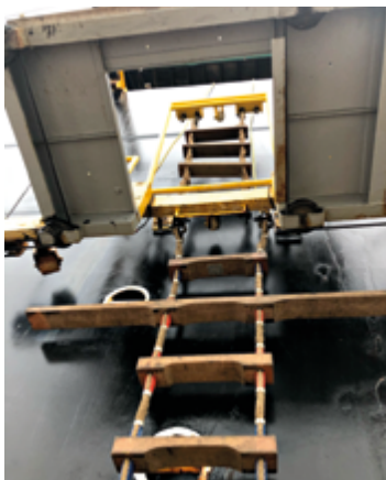
Figure 5. PBA as presented: Pilot ladder presented in two sections. Both sections are secured solely to the accommodation ladder platform instead of to the ship. Yellow horizontal frame sections are impeding access during ascent or descent.
