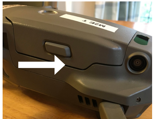
Figure 1 - Battery not clicked into place (note gap)
