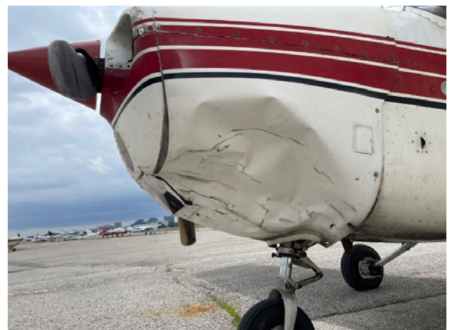
Damage to the Cessna 172 after collision with the DJI M210
