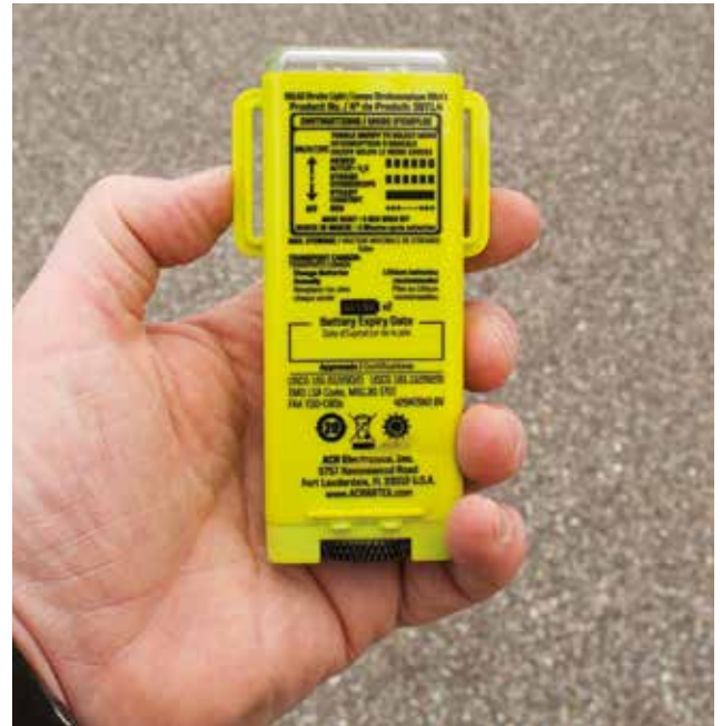
A typical personal locator beacon (PLB)
