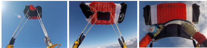
Images show a normal parachute opening with the uninhibited slider descending
