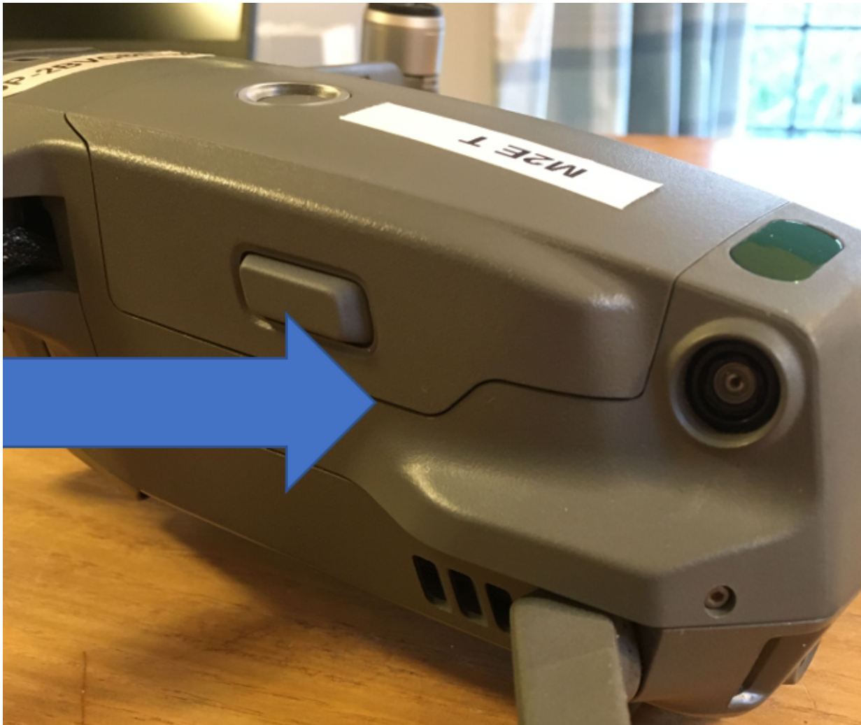
Figure 2 – Battery securely clicked into place (gap reduced)
