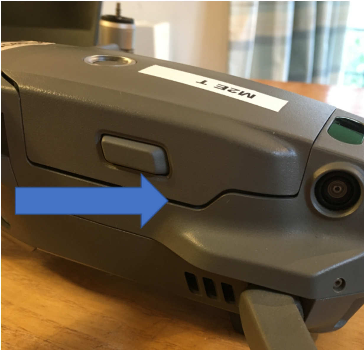
Figure 1 – Battery not clicked into place (note gap)
