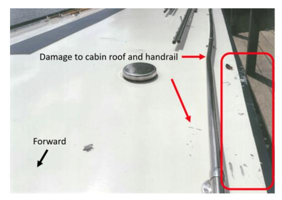
Damage to the Cabin roof and left side Handrail
